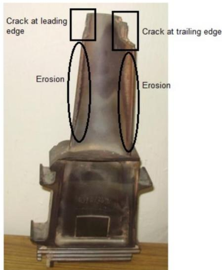
**Fig. 1 Blade Failure**
