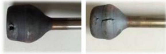
Fig. 6 Cracks in deformed surface
