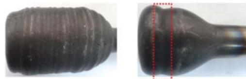
Generally, the preformed shape by electric upsetting should be controlled in a reasonable range, so as to ensure the forming quality of engine valves in final forming process. An inappropriate parameters combination in an electric upsetting process could result in unqualified shape or even lead to defects like external waviness and folding represented in Fig. 5.
