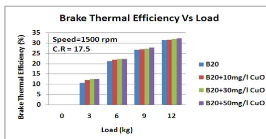
Fig.2 Load vs Brake thermal efficiency
