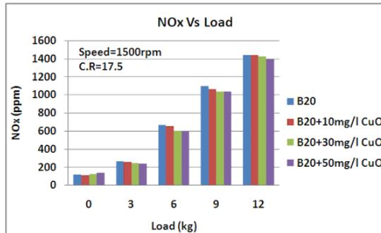
Fig.3 Load vs NO<sub>x</sub>
