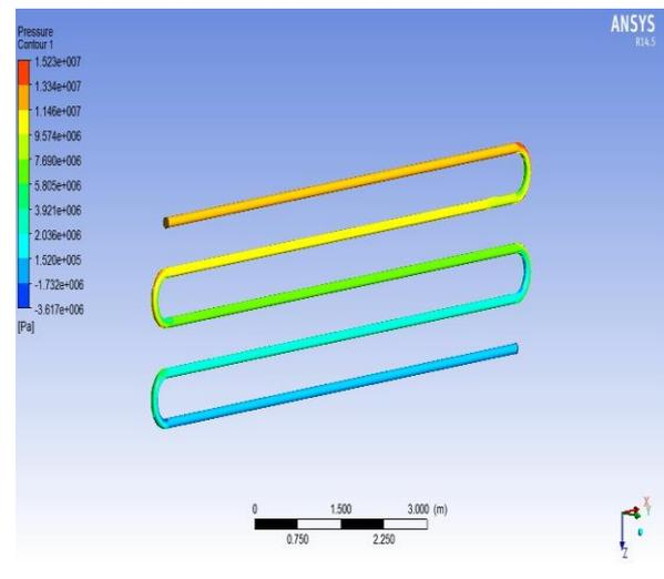
Fig.9 Pressure Distribution in wrought iron tubes
