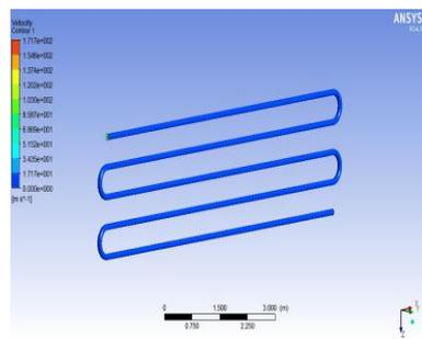
Fig.10 Velocity Distribution in wrought iron tubes
