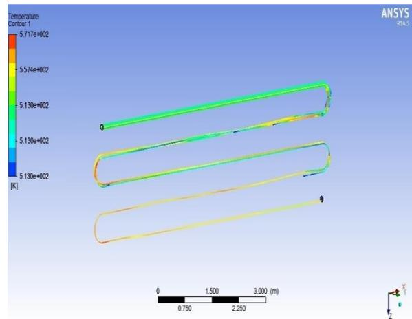
Fig.8 Temperature Distribution in wrought iron tubes
