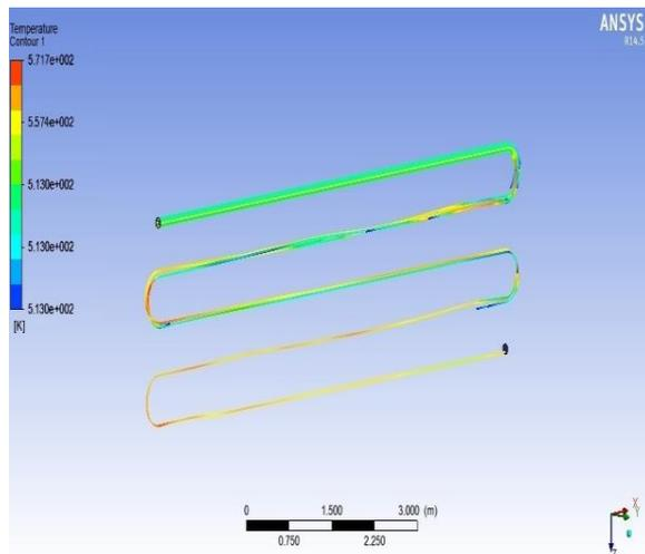
Fig.7 Temperature Distribution in carbon steel tubes
