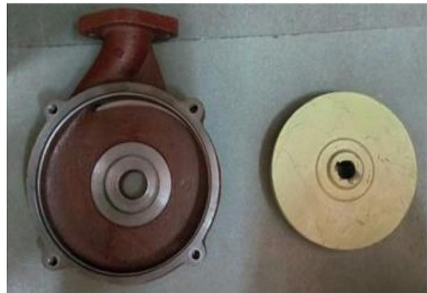
Fig.1 Casing and Impeller
