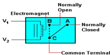
When a current flows through the coil, the resulting magnetic field attracts an armature that is mechanically linked to a moving contact. The movement either makes or breaks a connection with a fixed contact. When the current to the coil is switched off, the armature is returned by a
