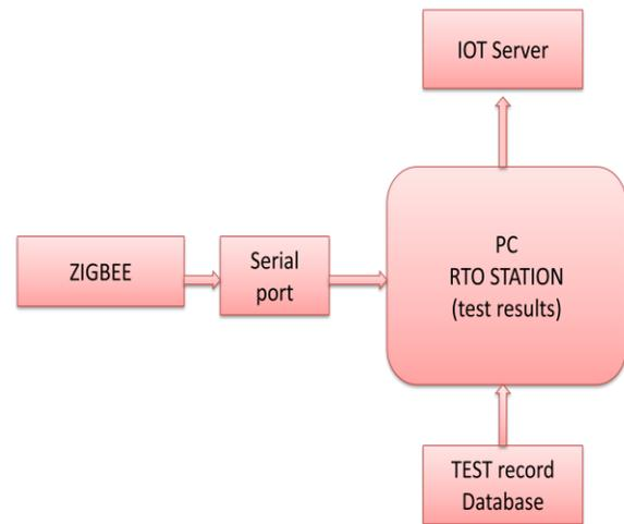
Fig.1.2 Block diagram for Receiver
