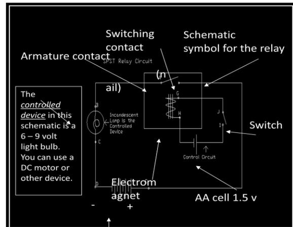
together the switch contact in the secondary circuit, thus supplying current to the component being operated.
