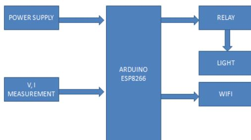
Block diagram of IoT based light controlling system
