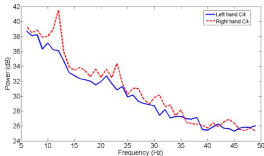
The solid (blue) line represents the spectrum on channel C4 averaged across all left hand trials. The dashed (red) line corresponds to the right hand trials. The trials display the biggest correlation with the labels around 12 Hz. It's also clear that the power is strongly attenuated in this frequency range for the left hand trials.
