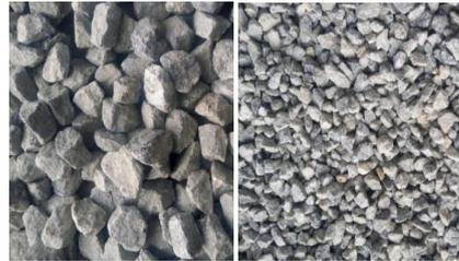
**Fig2.5.1 (20mm Aggregate & 12.5mm Aggregate)**
