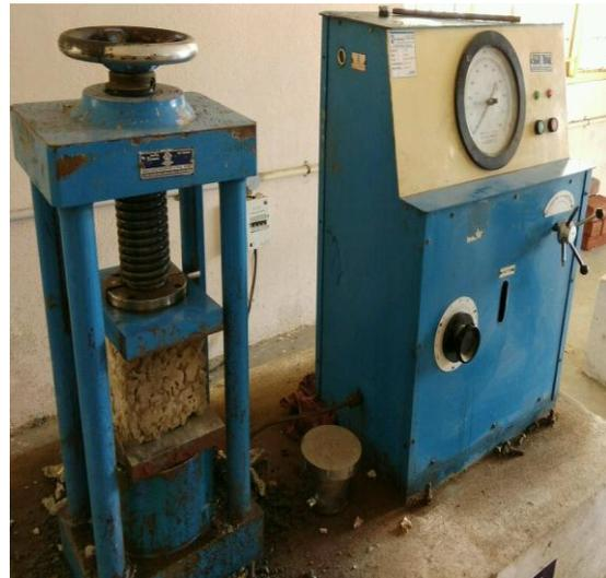
**Figure No 2:** Compressive test on cube
