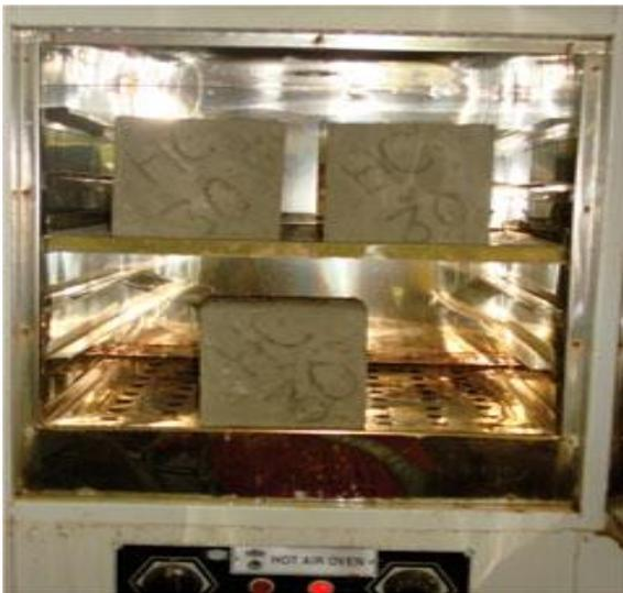
FIGURE 2: HOT CURING OF SPECIMENS
