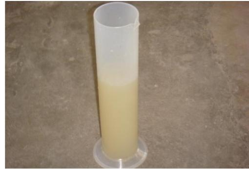
Sodium silicate is also known as water glass or liquid glass, available in liquid (gel) form. In present investigation sodium silicate 2.0 (ratio between Na<sub>2</sub>O to SiO<sub>2</sub>) is used. As per the manufacture, silicates were supplied to the detergent company and textile industry as bonding agent. Same sodium silicate is used for the making of geopolymer concrete.
