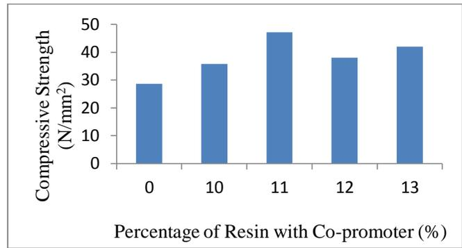
FIG. 1 COMPRESSIVE STRENGTH OF POLYMER CONCRETE
