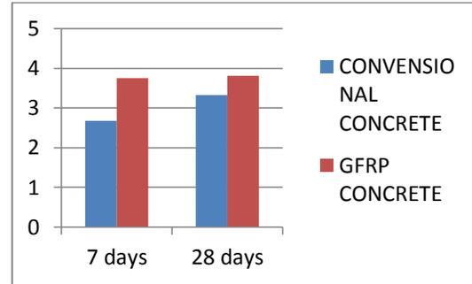
Fig 7 Graph Shows the Comparative of Flexural Strength Test Results
