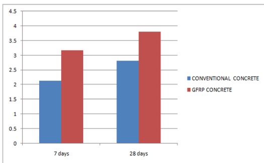
FIG 6 GRAPH SHOWS THE COMPARATIVE OF SPLIT TEST RESULTS
