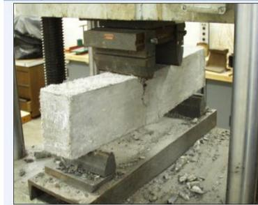
Fig 4 Flexural Strength Test
