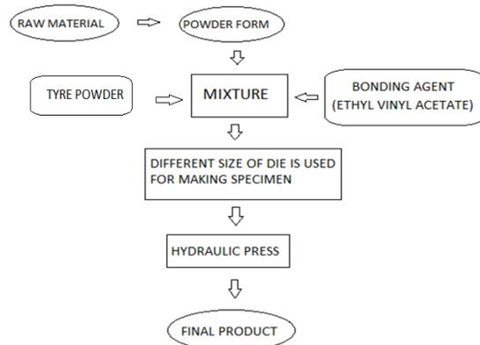
Fig.1: Procedure for preparing samples
