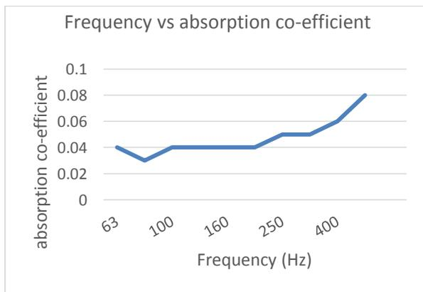
Graph 1: Frequency Vs absorption co-efficient of smaller mango specimen
