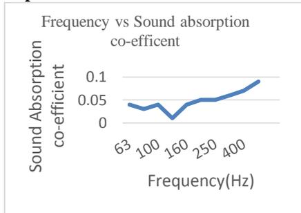
Graph 3: Frequency Vs absorption co-efficient of smaller neem specimen
