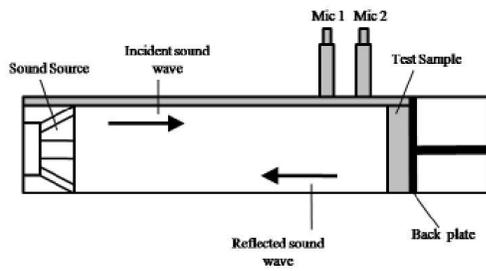
Fig.3: Impedance Tube Method
