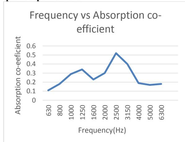
Graph 2: Frequency Vs absorption co-efficient of larger mango specimen
