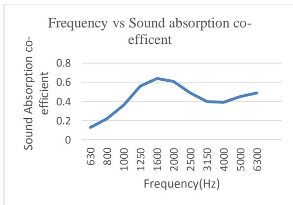
Graph 4: Frequency vs absorption co-efficient of larger neem specimen
