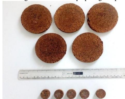
Fig.2: Specimen made for the test of Acoustic Properties
