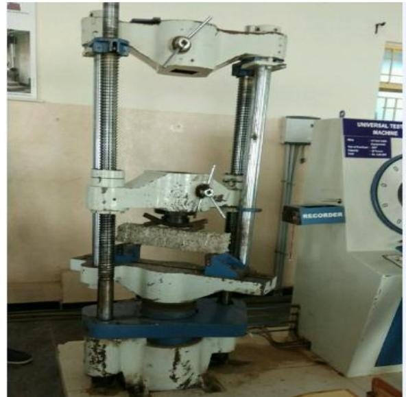
**Figure No:10 Flexural test on prism**
