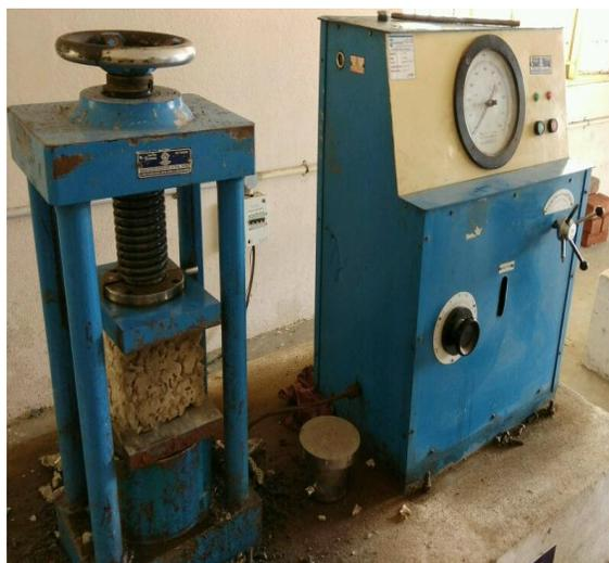
**Figure No2:** Compressive test on cube
