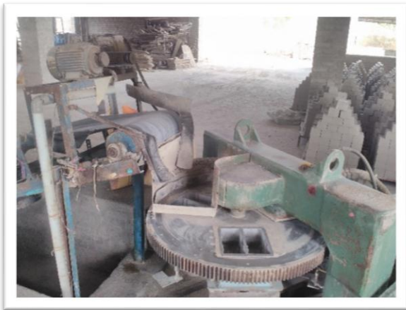
FIGURE 3: BRICK MOULDING MACHINE
