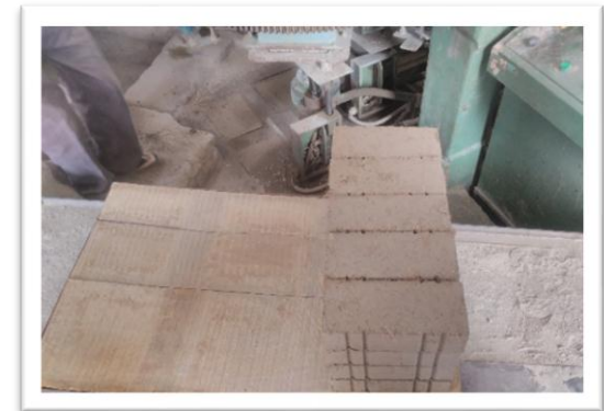
FIGURE 5: FLY ASH BRICKS WITH COIR FIBRE
