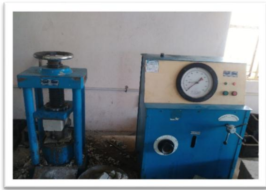
FIGURE 6: COMPRESSIVE STRENGTH TESTING MACHINE WITH BRICK
