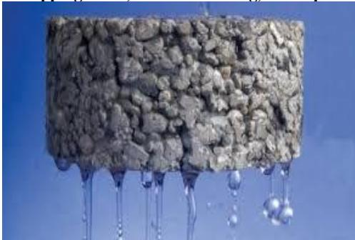
FIGURE - 1 PERVIOUS CONCRETE
