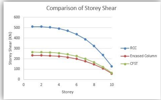
Fig.4.5 Comparison of Storey Shear for Seismic Zone 3
