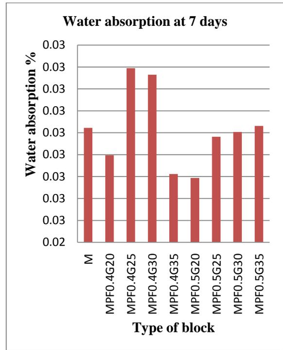
**Fig 4.2 Water absorption at 7 days for paver block without and with GGBS and fibres**
