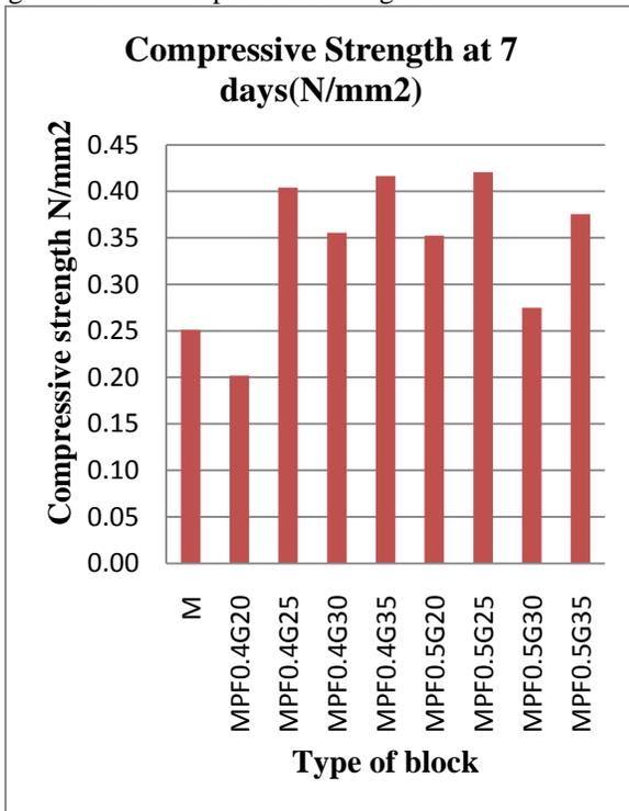
**Fig 4.1 Compressive strength at 7 days for paver block without and with GGBS and fibres**
