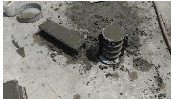
Figure 2.Casting of specimens
