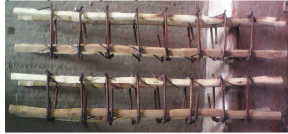
Fig 5: Treated Bamboo Reinforced Beam
