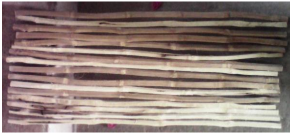
Fig.2. Bamboo for reinforcement
