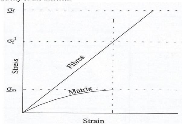
**Fig. 1:** High fibre content in a composite material
