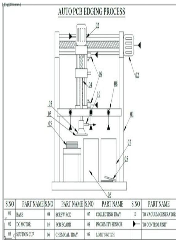
**Fig5. Automatic Etching Process**
