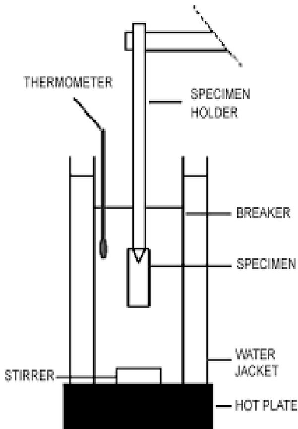
**Fig4. Manual Etching Process**
