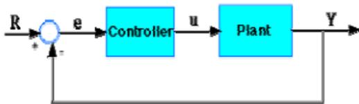
This signal (u) will be sent to the plant in (**milliliter**), and the new output (Y) will be obtained to **Tank 3**. This new output (Y) (**Flow**) from will be sent back to the sensor again to find the new error signal (e). The controller takes this new error signal and computes derivative and integral again. This process **goes open and closes the valve**.
