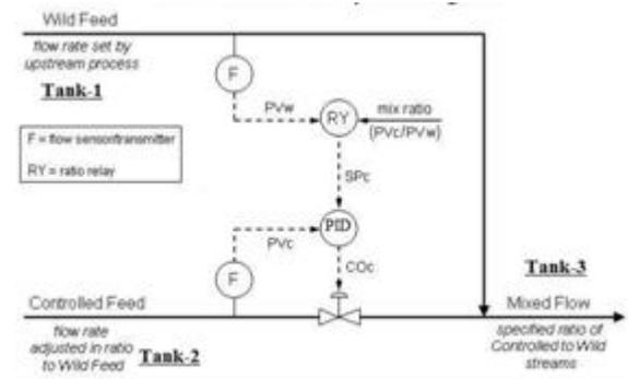
**Fig. 2 Ratio Control Conceptual Diagram**
