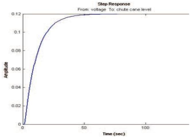
Fig.2: Open loop step response of crushing
