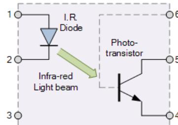
Fig 5. Phototransistor optocoupler circuit
