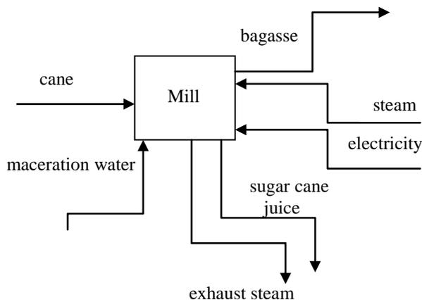
Fig.1: Block diagram of sugar input and output
