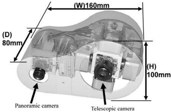
**Fig 1. Double Lens Tracking-Camera**
