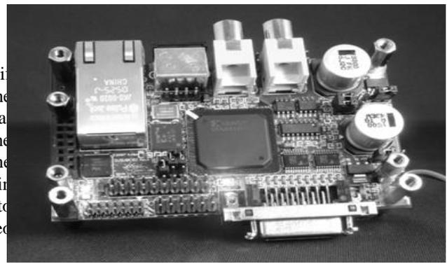
**Fig 2. FPGA Board**
