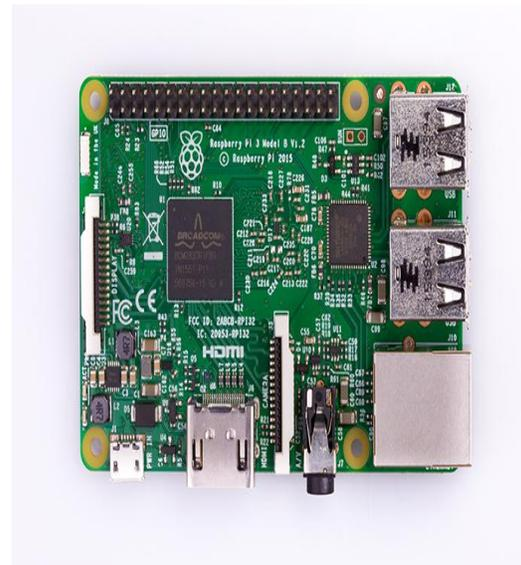
**Fig 3.2: Raspberry pi 3 model B+**
