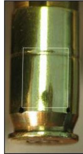
Cartridge case with an applied fingerprint
