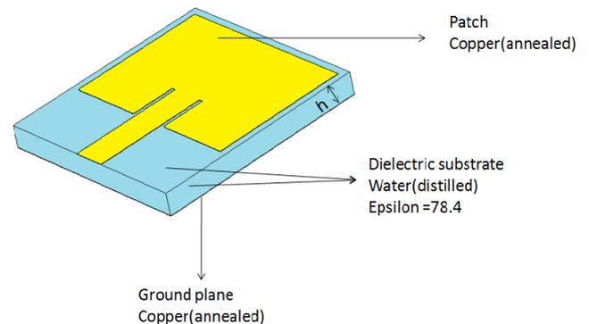
Fig1.(a).Structure of antenna
