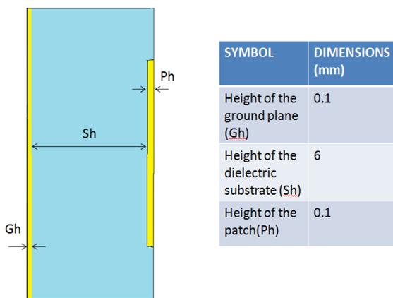
Fig1.(d).Side view of antenna
