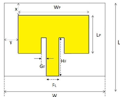
Fig1.(b).Top view of Antenna
