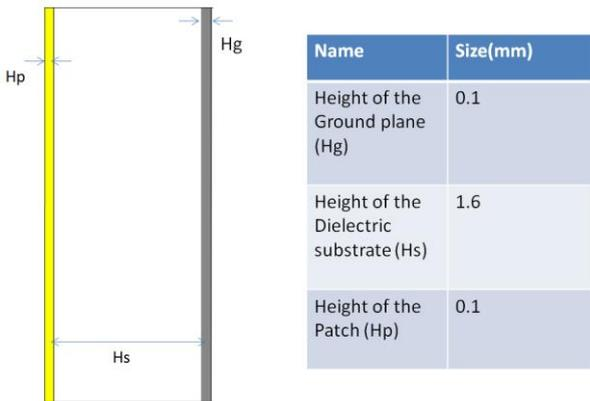
Fig1.(c).Side View Of The Antenna
