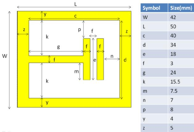
Fig1.(b).Top View Of The Antenna
