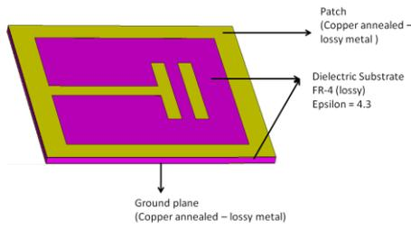
Fig1.(a).Structure Of The Antenna
