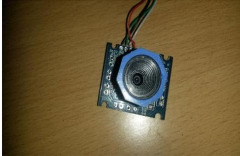
**Figure 4: IR Filter free Web Camera**
