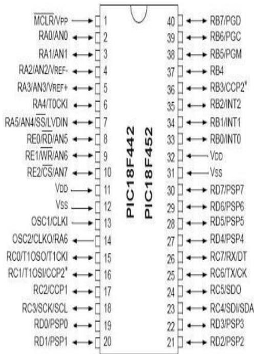
Figure 5. Pin Diagram
