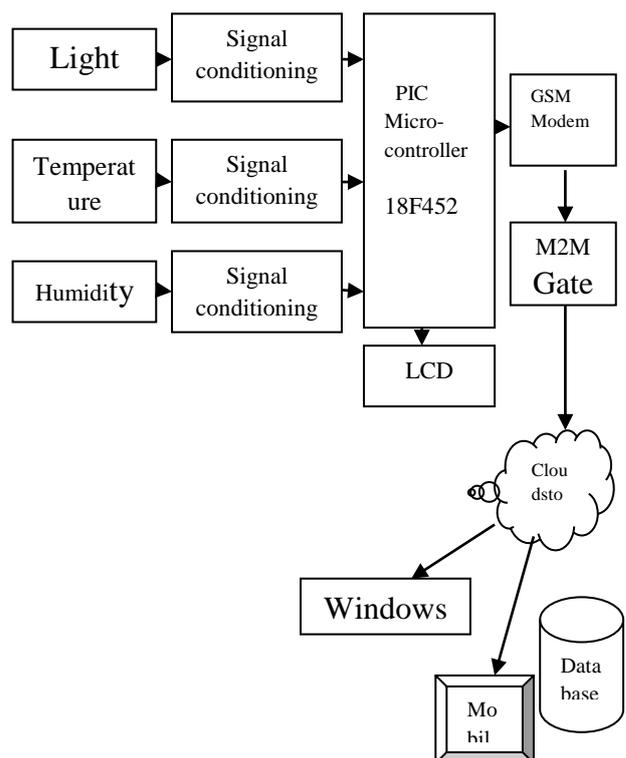
**Figure 3.** Block diagram Of Industrial Monitoring Using M2M
