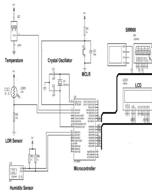
**Figure 4.** Circuit diagram of server room environmental monitoring system
