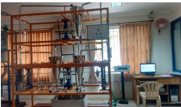
Fig. 1 Experimental Setup of Conical Tank System
