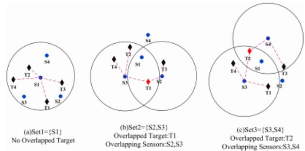
**Figure.3.Overlapped target and overlapping sensors in joint set**
