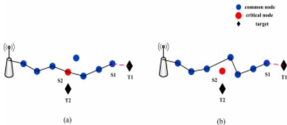
**Figure.2. Avoid traversing a node that covers a critical target**
