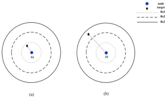
Figure.4. one node, one target and three power levels.
