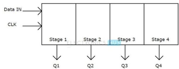
The clear (CLR) signal is connected in addition to clock signal to all the 4 flip flops in order to RESET them and the serial data is connected to the flip flop at either end (depending on shift left register or shift right register). The output of the first flip flop is connected to the input of the next flip flop and so on. All the flip flops are connected with a common clock.
