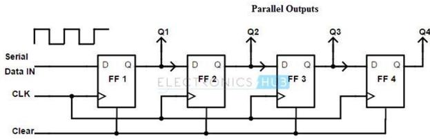
Unlike the serial in serial out shift registers, the output of Serial in Parallel out (SIPO) shift register is collected at each flip flop. Q1, Q2, Q3 and Q4 are the outputs of first, second, third and fourth flip flops, respectively. The main application of Serial in Parallel out shift register is to convert serial data into parallel data. Hence they are used in communication lines where demultiplexing of a data line into several parallel line is required.
