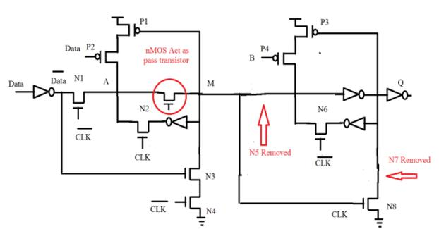
Fig.2.Restructured D Flip-Flop
