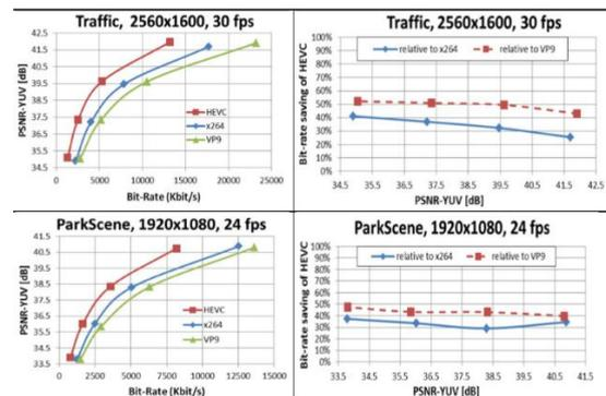
**FIGURE 6.7.1 R-D CURVES AND CORRESPONDING BIT-RATE SAVING PLOTS FOR SEVERAL TYPICAL EXAMPLES OF TESTED SEQUENCES.**
